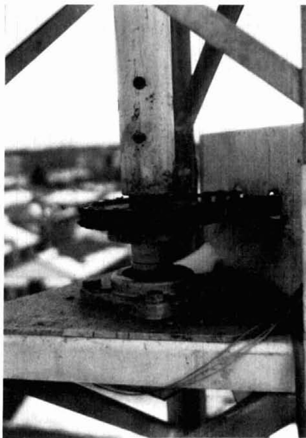
fig. 3. Completed mast assembly consists of chain drive steel pin and flanged cartridge.
